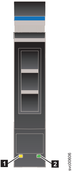
Figure 11. LED indicators on a single 2.5 inch drive
