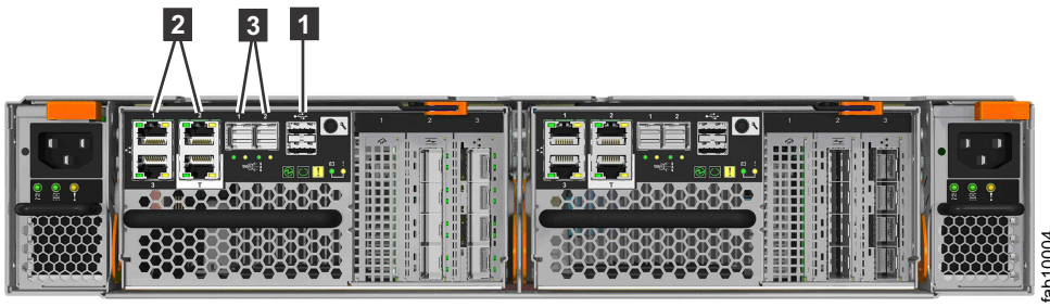
Figure 21. Storwize V7000 2076-524 node canister ports
