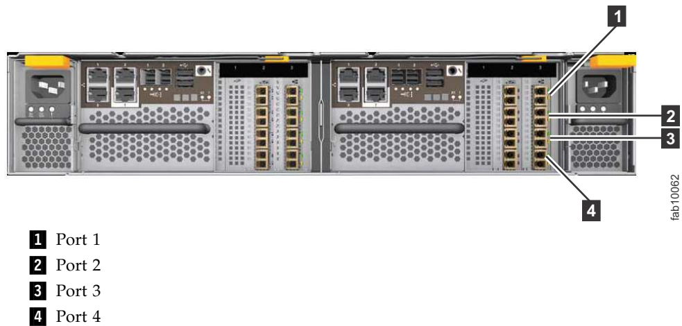
Figure 26. 10 Gbps Fibre Channel over Ethernet/iSCSI host interface adapter ports
